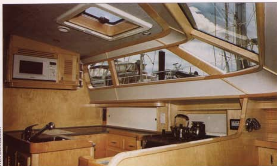
Waterline's interiors are fit out to a high standard. Left —Mettle's galley, located under the pilothouse. Steel construction allows the support structure for the windows to be relatively light. Right —A maple sunburst-pattern table with inlaid cherry border.
