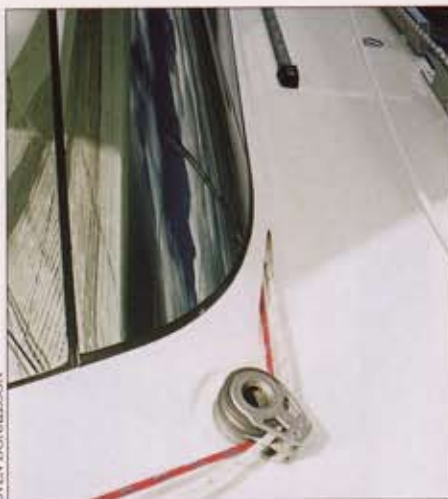
Left —The ½" (13mm) laminated safety glass has a reflective coating to reduce solar heating. Note the metalwork details on deck: hidden conduits for the lines, and polished stainless steel toerails. Right —The yard has so far built two motoryachts. Shown here is Ted K, designed by Steve Seaton. The concave topsides and bulbous bow involved some of Waterline's most difficult steelwork to date. The art on the bulb is by David Tolman, an employee at the yard.
