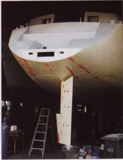
Left —Steelwork complete, a Waterline 46 is moved from the metal shop to the finishing shop. Right —Rutherford's sailboat designs favor semi-balanced rudders supported by a partial skeg.
