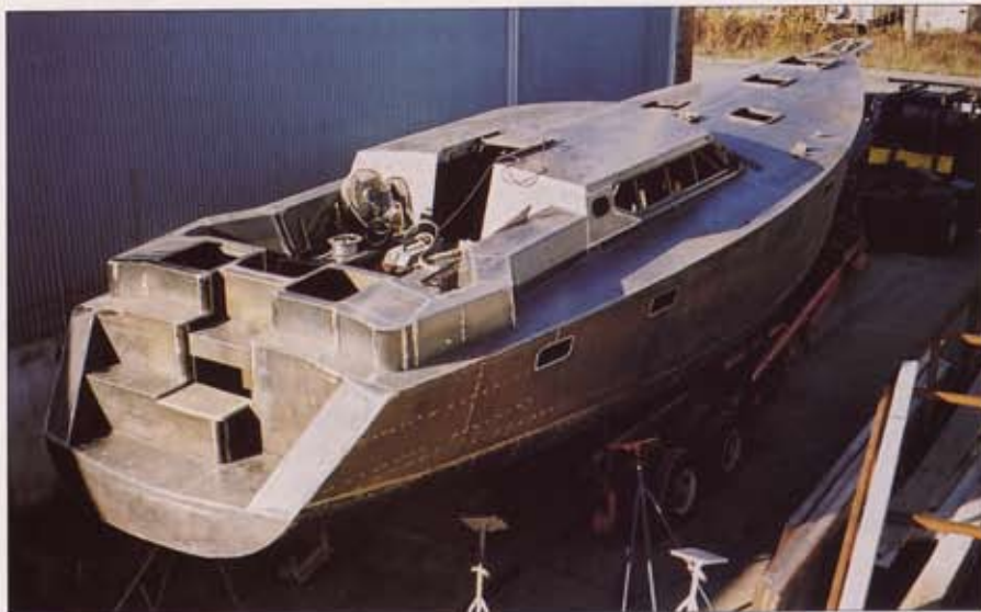
Left —Steelwork complete, a Waterline 46 is moved from the metal shop to the finishing shop. Right —Rutherford's sailboat designs favor semi-balanced rudders supported by a partial skeg.
